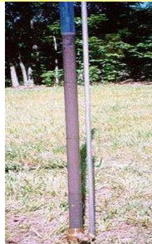
After removing, measure from the bottom of the rod to the top of the sludge layer
