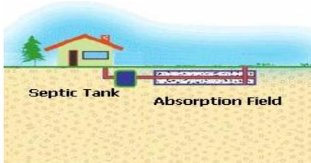
The subsurface sewage treatment system is the most common on-site wastewater treatment method. Approximately 60% of the soils in Oklahoma are suitable for this type of treatment method. Subsurface sewage treatment system consists of a septic tank and an absorption field made up of a series of shallow trenches called lateral lines. When subsurface sewage treatment systems are properly designed, operated and maintained, the wastewater will receive proper treatment before it enters the environment.
