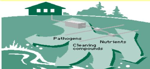
A subsurface absorption field is made up of a series of shallow trenches called lateral lines. Lateral lines can be comprised two ways: **(1)** consist of perforated pipe surrounded on all sides by storage media (gravel or tire chips) and back-filled with native soil; or **(2)** leaching chambers that do not contain media. As the effluent slowly trickles through the perforated
